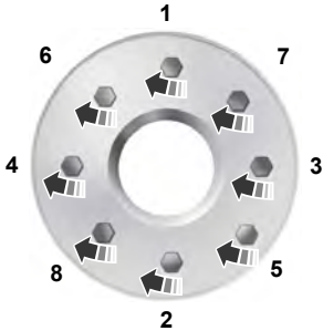
8-lug nut torque sequence
