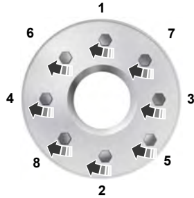
8-lug nut torque sequence
