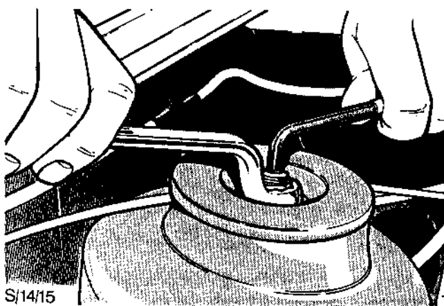
Fig.2. The 6mm hexagonal key to hold strut on removal and installation of top mount nut.
